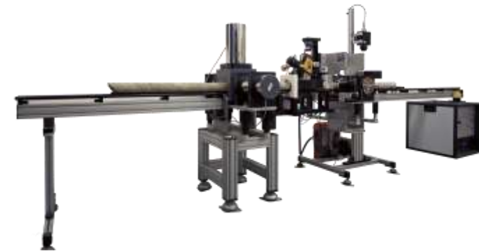
MSCL-S with 9 sensors incl. XRF
